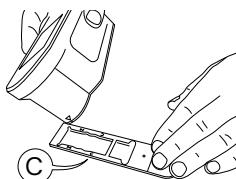
3. Fix the macsReader on the stencil **in position 'C'**.
