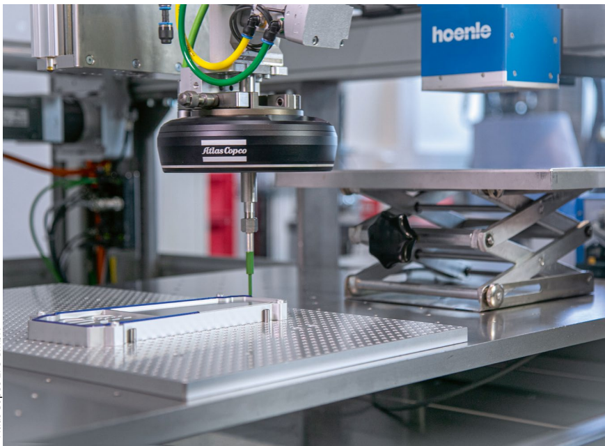
High-speed dispensing system with a single-component dispenser for serial sealing applications.
