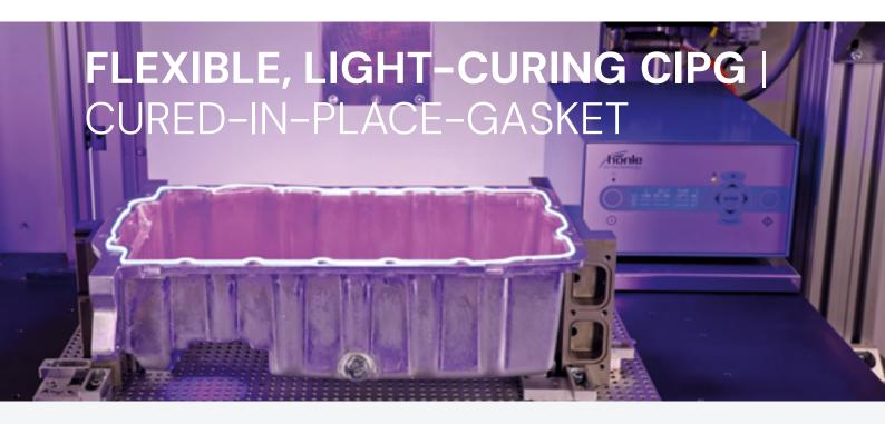
Liquid gaskets offer a simple and effective solution for sealing even complex 3D geometries that conventional gaskets cannot reliably seal.
