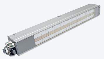
The LED Powerline LC HV is a high-performance UV-LED array for intermediate curing (pinning) and final curing at printing applications. Other application fields are the curing of varnishes or UV reactive adhesives and pottings. Power is supplied via 400 V DC. Separate regulation of each LED segment, e.g. for format size control.
