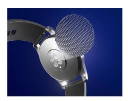
Caption: The new UV adhesive Vitralit® UC 1633 is used for microlenses on smart watch sensors
